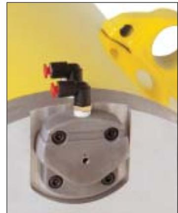
**Z Stop:** The optional Z Stop is a patent pending device that will eliminate the down-drift of suspended loads or tools during shut down or at night when the air supply is shut off. The Z Stop will stop drift within 6 inches (152.4 mm) and put the Balance Air into a mechanically locked position preventing damage to tools or objects below the suspended load. Available for use on all 10 inch (254 mm) diameter units.
