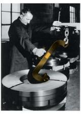
Placing spacer blocks between stacked coils permits easy insertion of the wedge. Lightweight and pivoting wedge makes it easy to position the hook.
