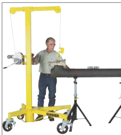
Position fittings with Sumner Adjust-A-Fit™
