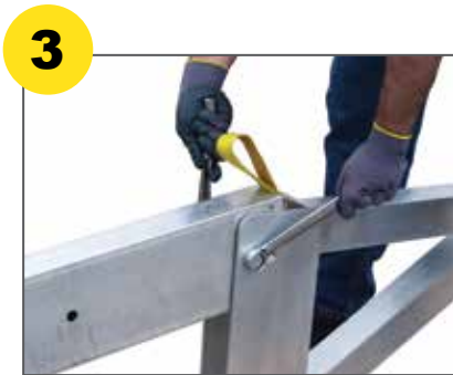
Attach with one bolt to each "A" Frame
