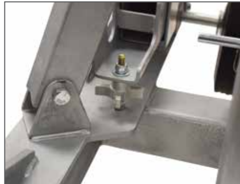
Adjustment base leveling screw to accommodates base extensions on unlevel floors.
